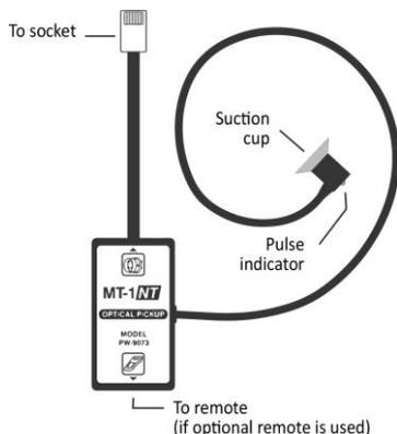
Fig. 2.5a – Optical Pickup
