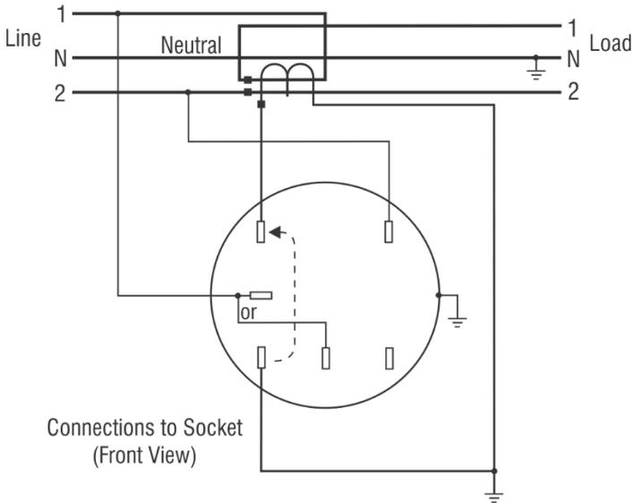
Form 3S single-phase, 120 volts two-wire with CT is also compatible.
