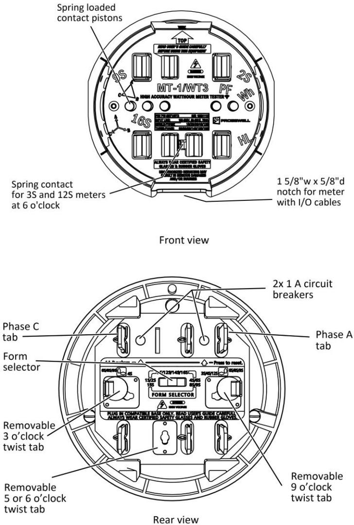
**Fig. 2.1 – Front and Rear View of the Socket**
